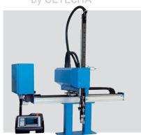
GL 1 and GL 3 remove sprues and small parts from small- and medium-sized injection molding machines quickly and reliably. Communication with the injection molding machine takes place via the Europmap interface. With three independent, linear servoaxes, the machine sticks to the job with exact positioning capability and reproducibility.
